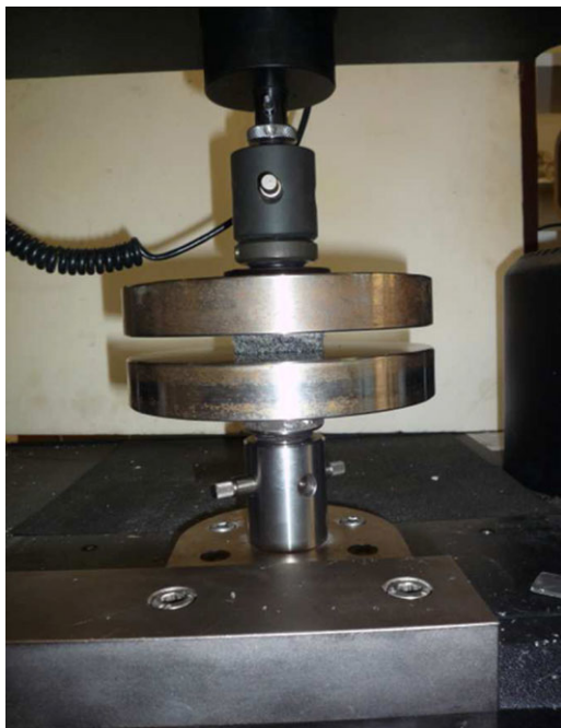
Figure 4. Sample of polyurethane foam under compression stress. [Color figure can be viewed in the online issue, which is available at wileyonlinelibrary.com .]
